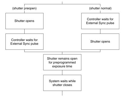
Figure 17. Chart Showing Two External Sync Timing Options
